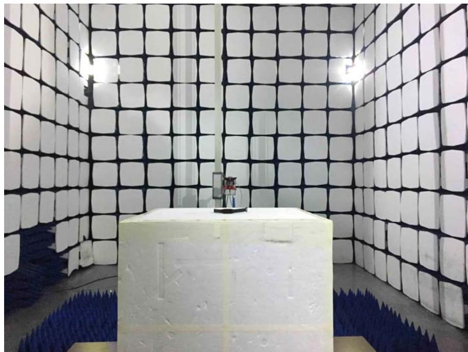
**Radiation Emission View (Above 18GHz)**
