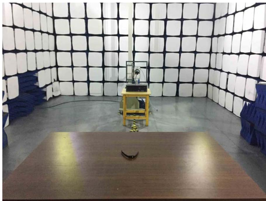
**Radiation Emission Test Setup (30MHz to 1GHz)**
