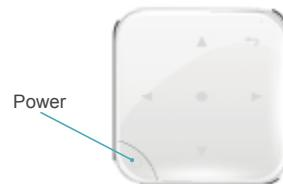
1.Click and hold the power button for 5 seconds to turn on or off the projector
