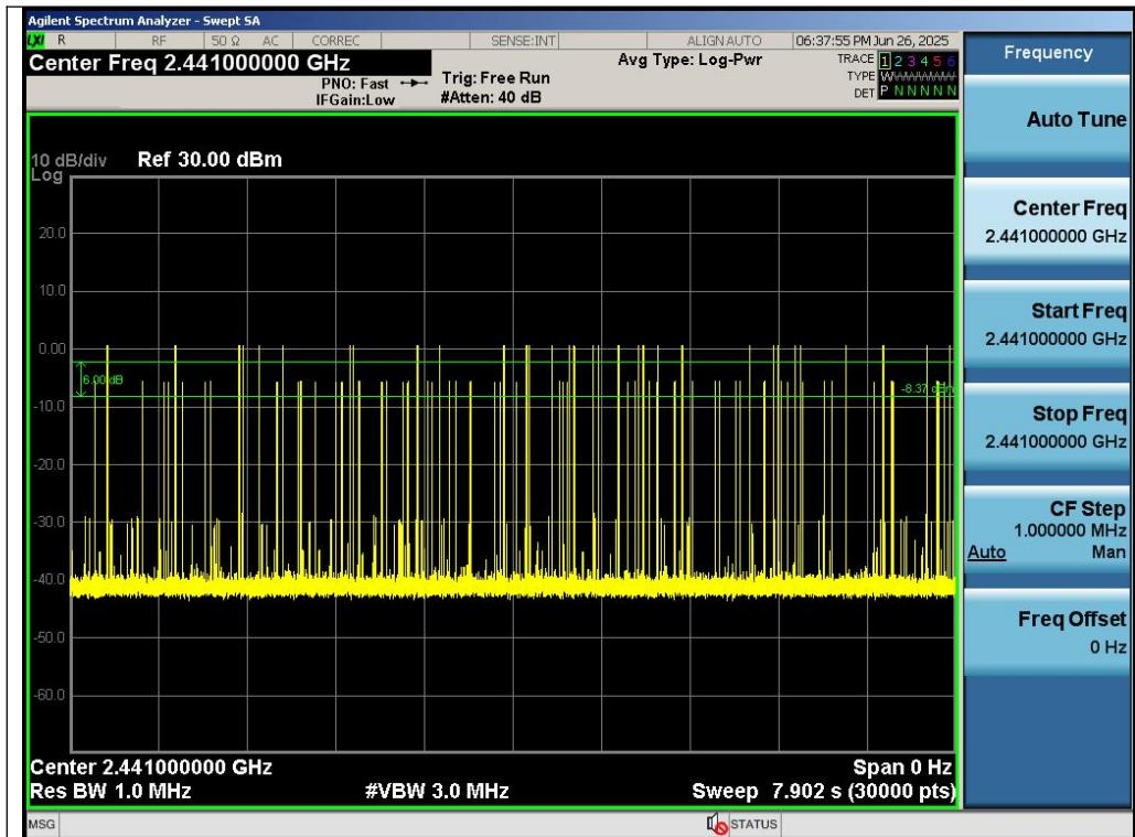
Test\_Graph\_EDR\_HOP\_ANT1\_NA\_3Mbps\_2441\_Number of Bursts
