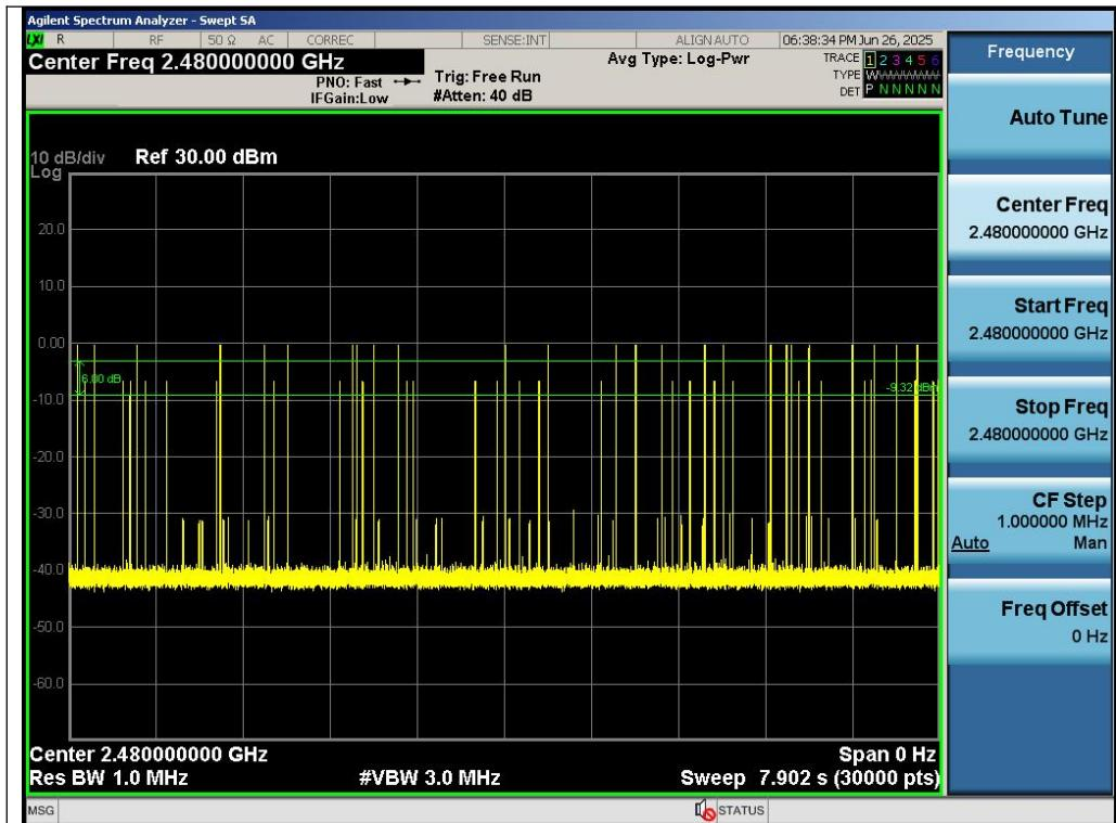
Test\_Graph\_EDR\_HOP\_ANT1\_NA\_3Mbps\_2480\_Number of Bursts
