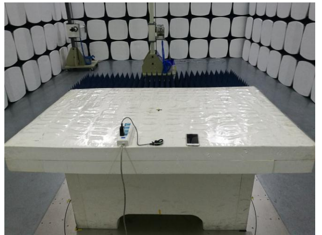
Radiated Spurious Emissions Test Setup Above 1GHz
