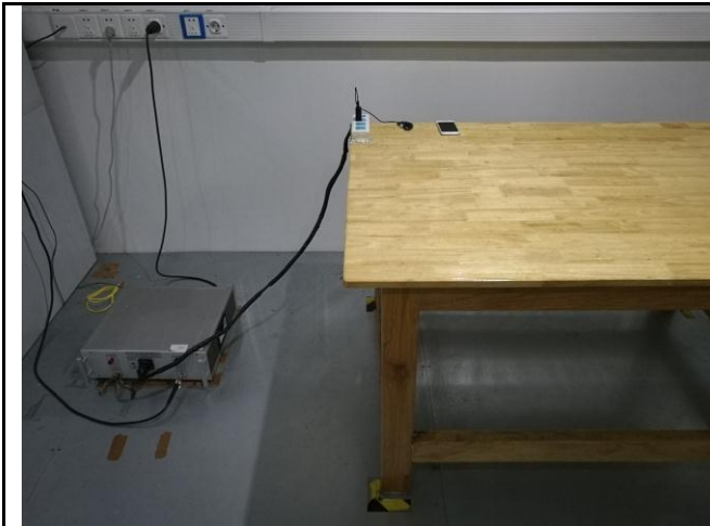
Conducted Emissions Test Setup Front View
