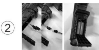
Docking the rechargeable battery cable, and put it into the battery compartment.
