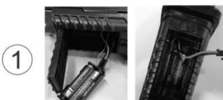
Install two AAA batteries into the battery compartment according to the positive and negative instructions.
