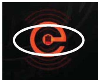
The batteries in the Redi-Temp Electronic System valves should be replaced when the battery icon in the application turns red.
