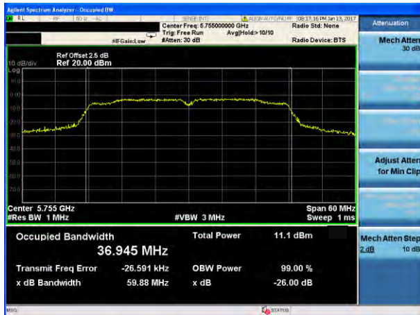
(802.11ac40) -26dB&99% Bandwidth plot on channel 151
