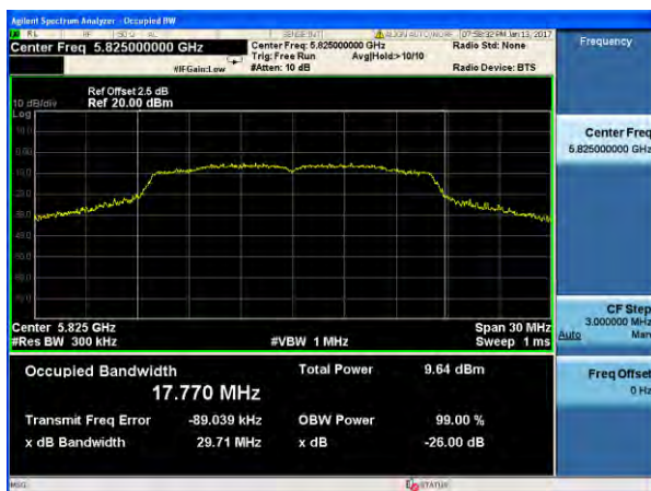
(802.11a) -26dB&99% Bandwidth plot on channel 165
