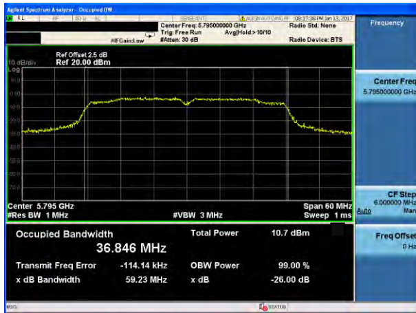
(802.11ac40) -26dB&99% Bandwidth plot on channel 159
