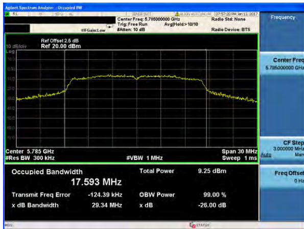
(802.11a) -26dB&99% Bandwidth plot on channel 165
