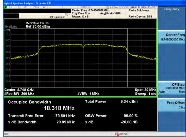
(802.11n20) -26dB&99% Bandwidth plot on channel 157
