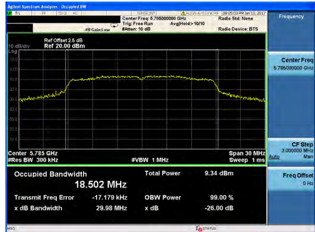
(802.11n20) -26dB&99% Bandwidth plot on channel 165
