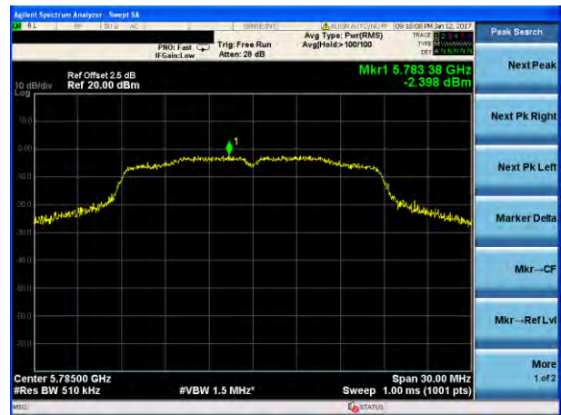
(802.11n20) PSD plot on channel 165
