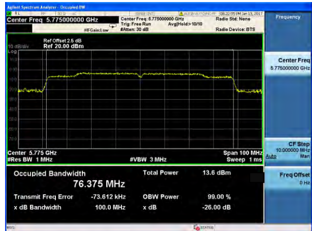
(802.11ac80) -26dB&99% Bandwidth plot on channel 155
