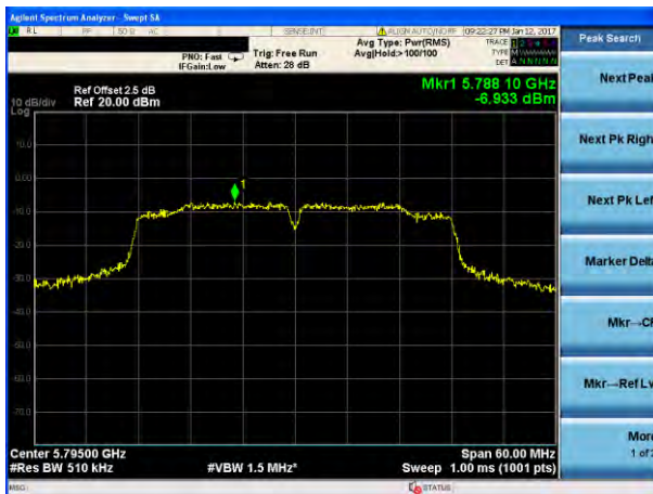
(802.11n40) PSD plot on channel 159
