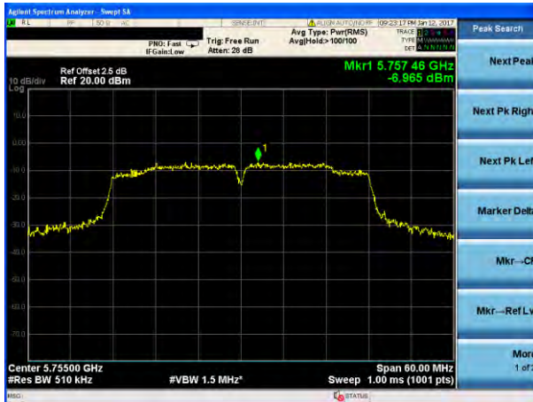
(802.11n40) PSD plot on channel 151
