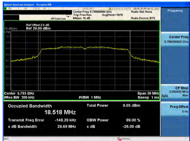
(802.11ac20) -26dB&99% Bandwidth plot on channel 165
