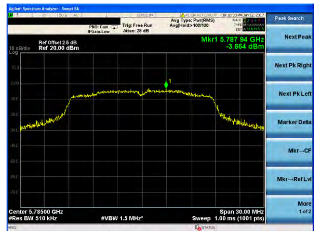
(802.11ac20) PSD plot on channel 157
