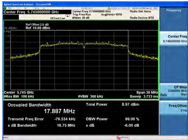
(802.11ac20) -6dB Bandwidth plot on channel 157
