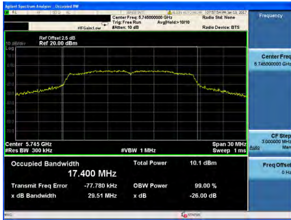
(802.11a) -26dB&99% Bandwidth plot on channel 157
