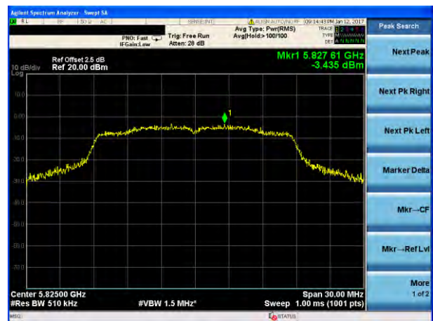
(802.11n20) PSD plot on channel 165
