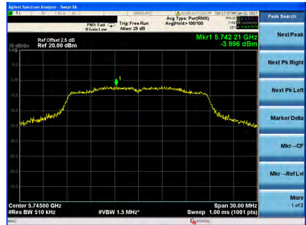
(802.11ac20) PSD plot on channel 149
