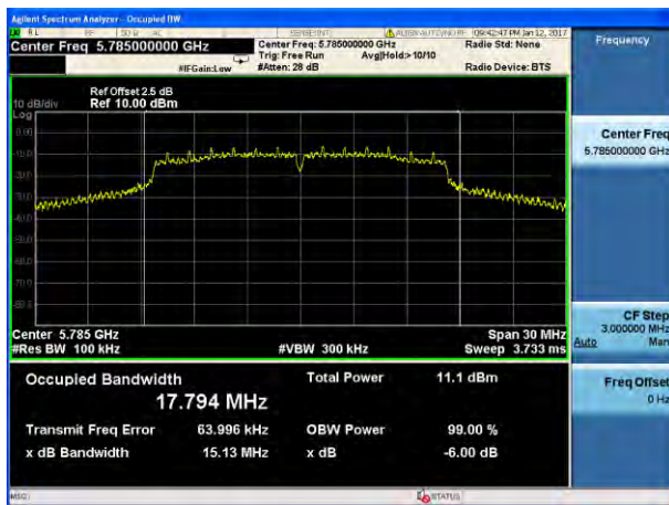
(802.11a) -6dB Bandwidth plot on channel 165
