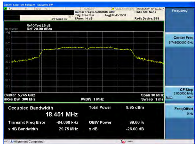
(802.11ac20) -26dB&99% Bandwidth plot on channel 157
