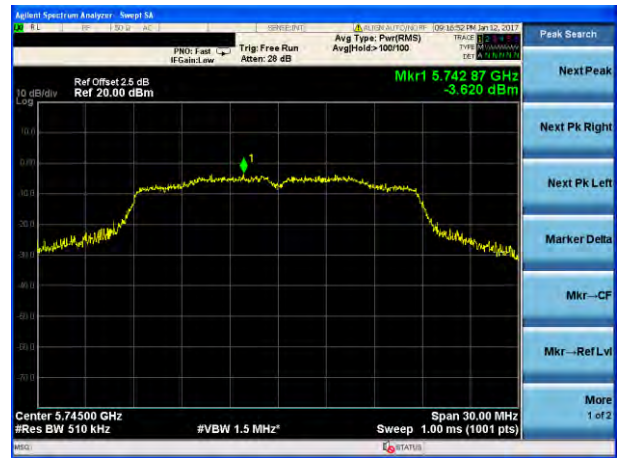
(802.11n20) PSD plot on channel 157
