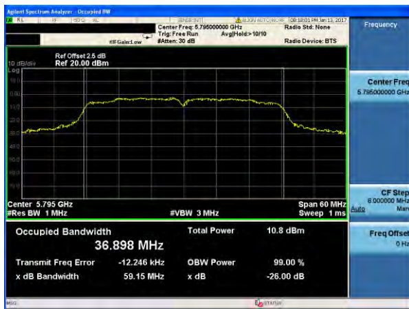
(802.11n40) -26dB&99% Bandwidth plot on channel 159
