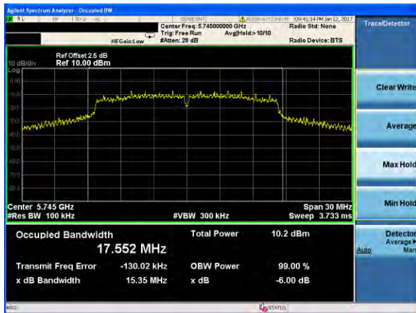
(802.11a) -6dB Bandwidth plot on channel 157
