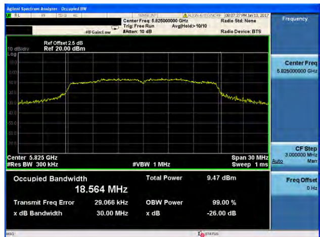
(802.11ac20) -26dB&99% Bandwidth plot on channel 165
