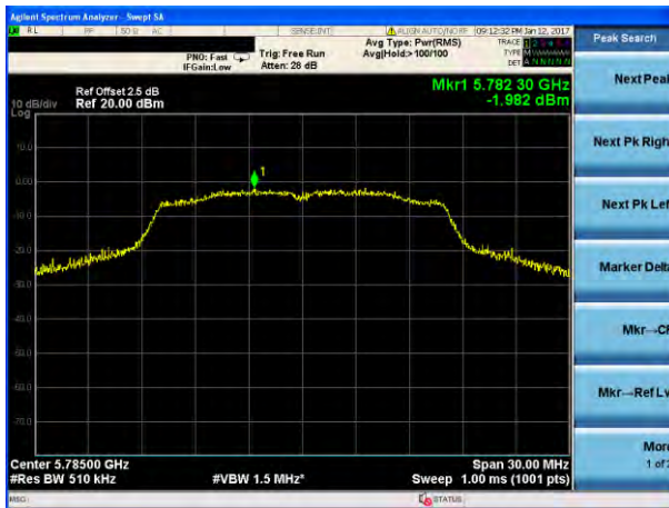
(802.11a) PSD plot on channel 165
