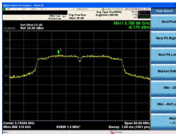
(802.11ac40) PSD plot on channel 159
