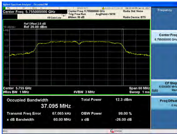
(802.11n40) -26dB&99% Bandwidth plot on channel 159
