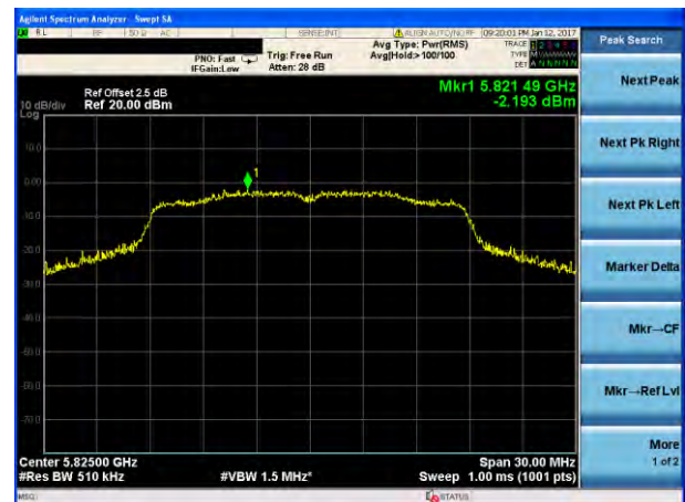
(802.11ac20) PSD plot on channel 165
