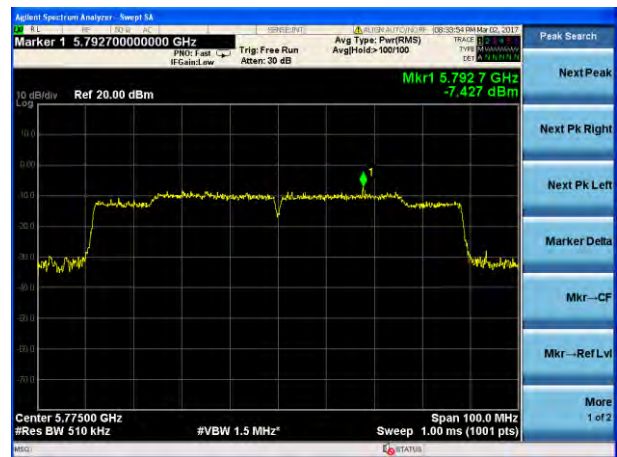
(802.11ac80) PSD plot on channel 155
