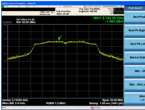
(802.11a) PSD plot on channel 157
