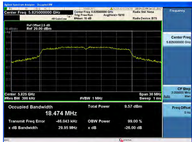
(802.11n20) -26dB&99% Bandwidth plot on channel 165
