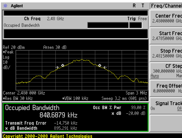
20dB Bandwidth plot on channel 78 (1Mbps)
