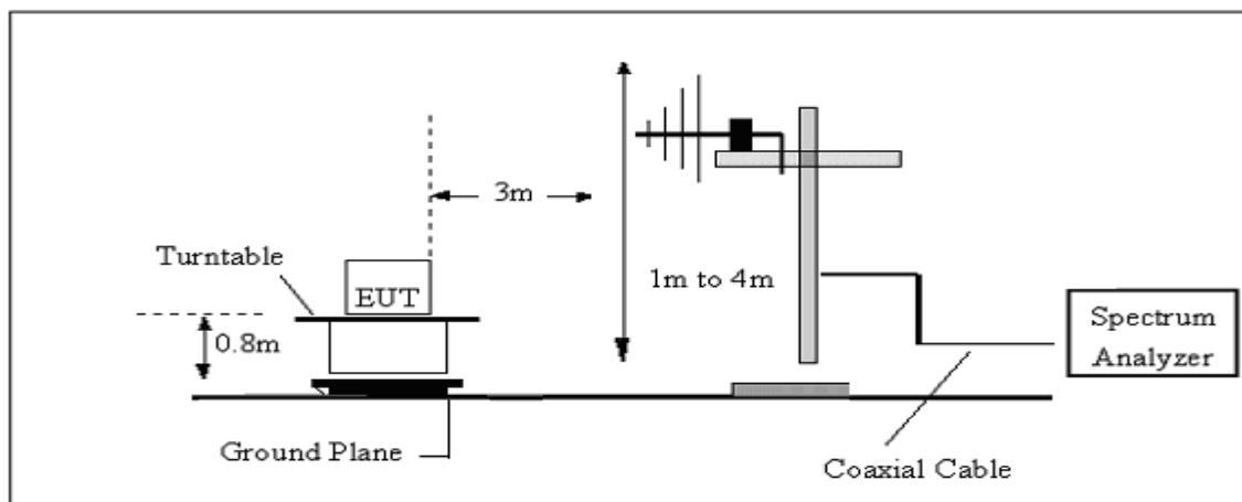
(B) Radiated Emission Test-Up Frequency Above 1GHz
