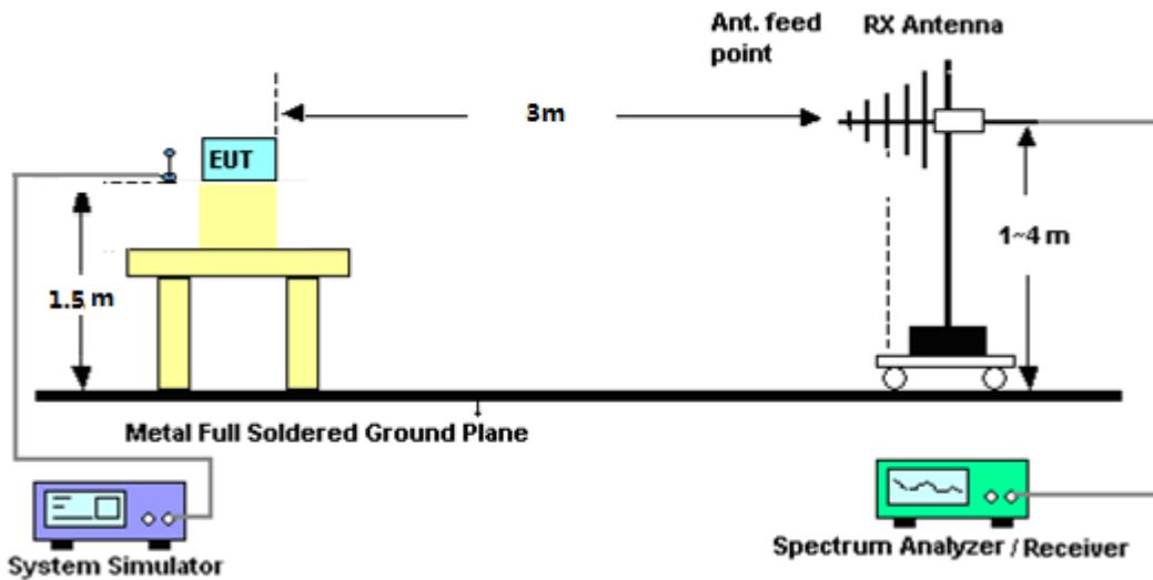
For radiated test from above 1GHz
