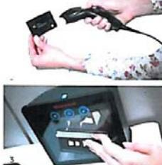
The bar code is transmitted by LED on the front of the card. To read a barcode from the Cardberry place the scanner's laser beam to the LED on the card (Figure 2). If the barcode scanner is omnidirectional (Figure 3), the Cardberry card must be closely attached to the scanner's glass.
