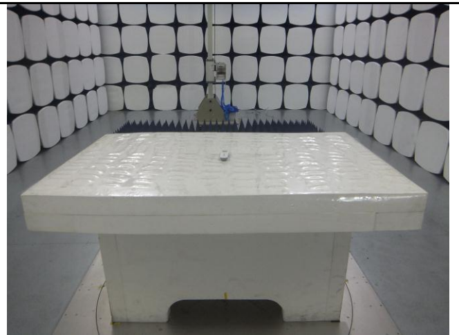
Radiated Emissions Test Setup Above 1GHz
