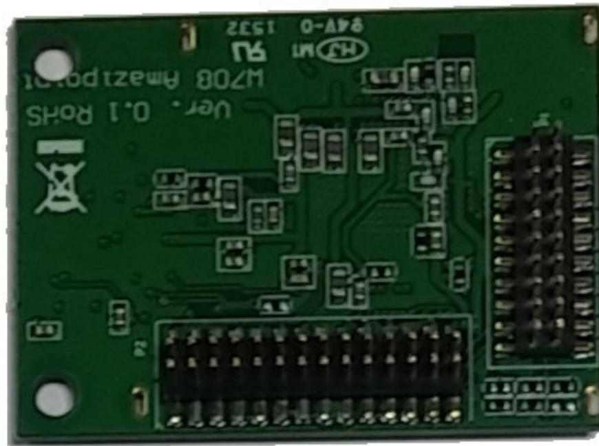
There are two 1.27mm pitch header on the bottom side of module P1 and P2.
