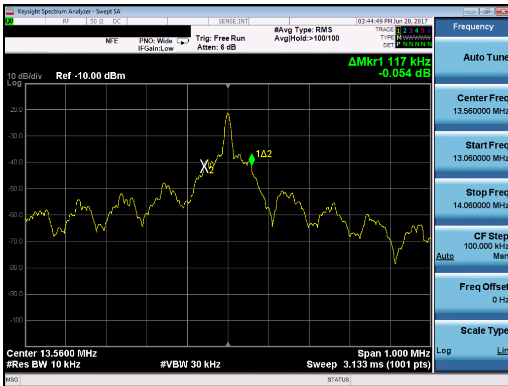
Figure 7-4. 20dB Bandwidth Plot (160132-915)
