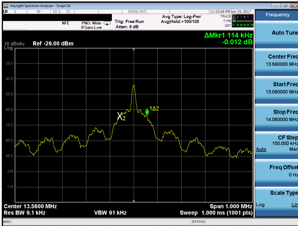
Figure 7-3. 20dB Bandwidth Plot (160143-915)
