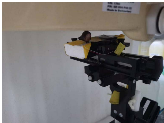
Fig-4.2 Top of EUT with 0 cm Gap (Head Mode)
