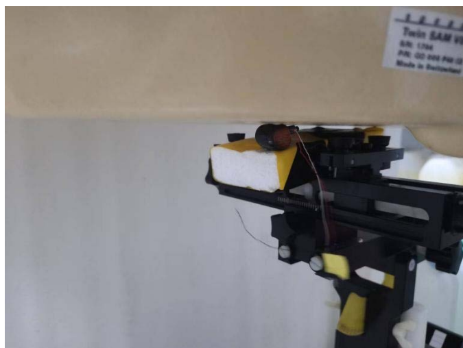
Fig-4.4 Right Side of EUT with 0 cm Gap (Head Mode)
