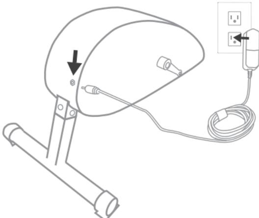
NOTE: it may take up to 2 hrs for Cycli to be fully charged. You can check the battery status icon on Cycli's built in touch screen:
