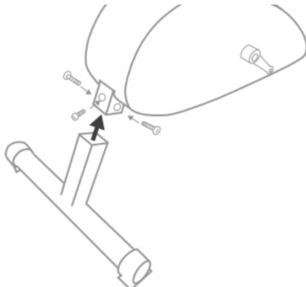
2. Use the screws to attach the Front Leg to the Cycle Case.
