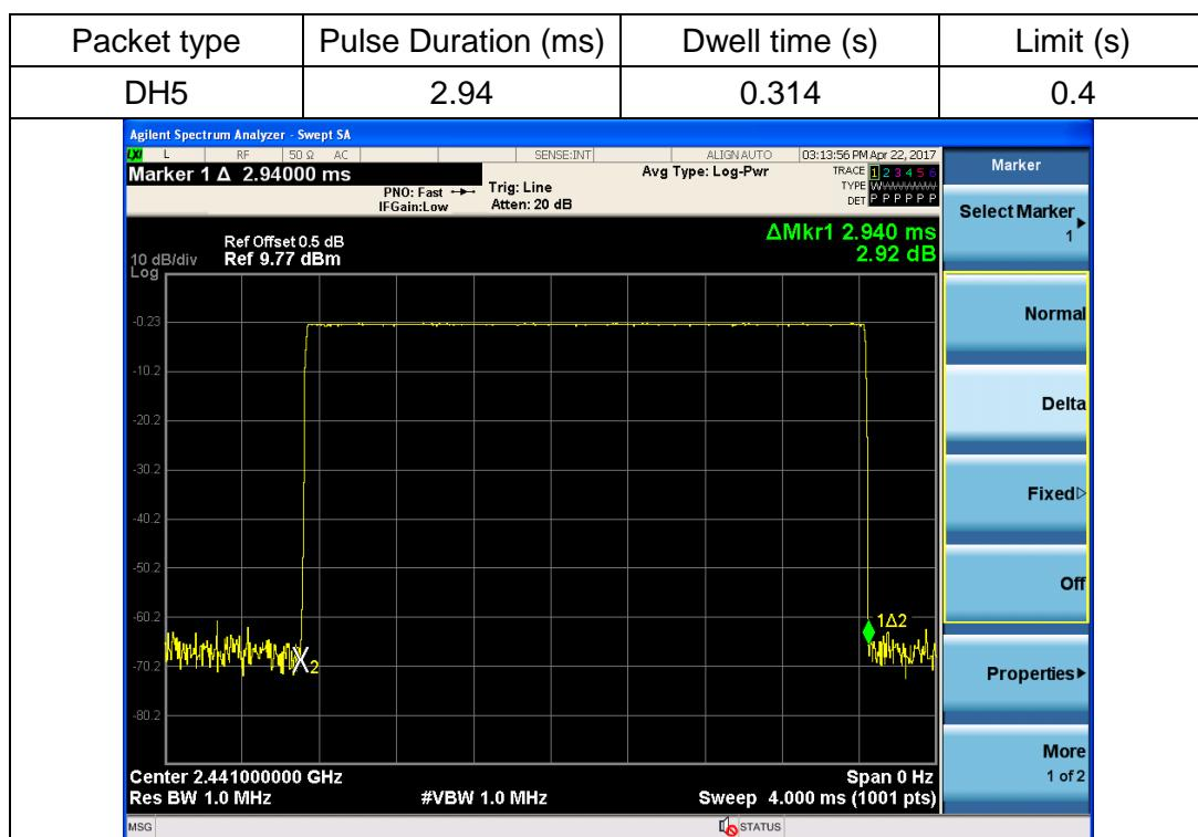
Note: for the worst mode of DH5 packet type, in normal hopping mode, hopping rate is 1600hops/s with 6 slots in 79 hopping channel
