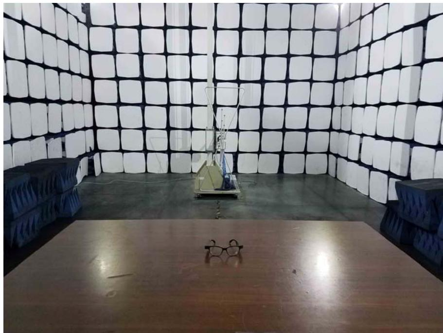
**Radiation Emission Test Setup (Above 1GHz)**
