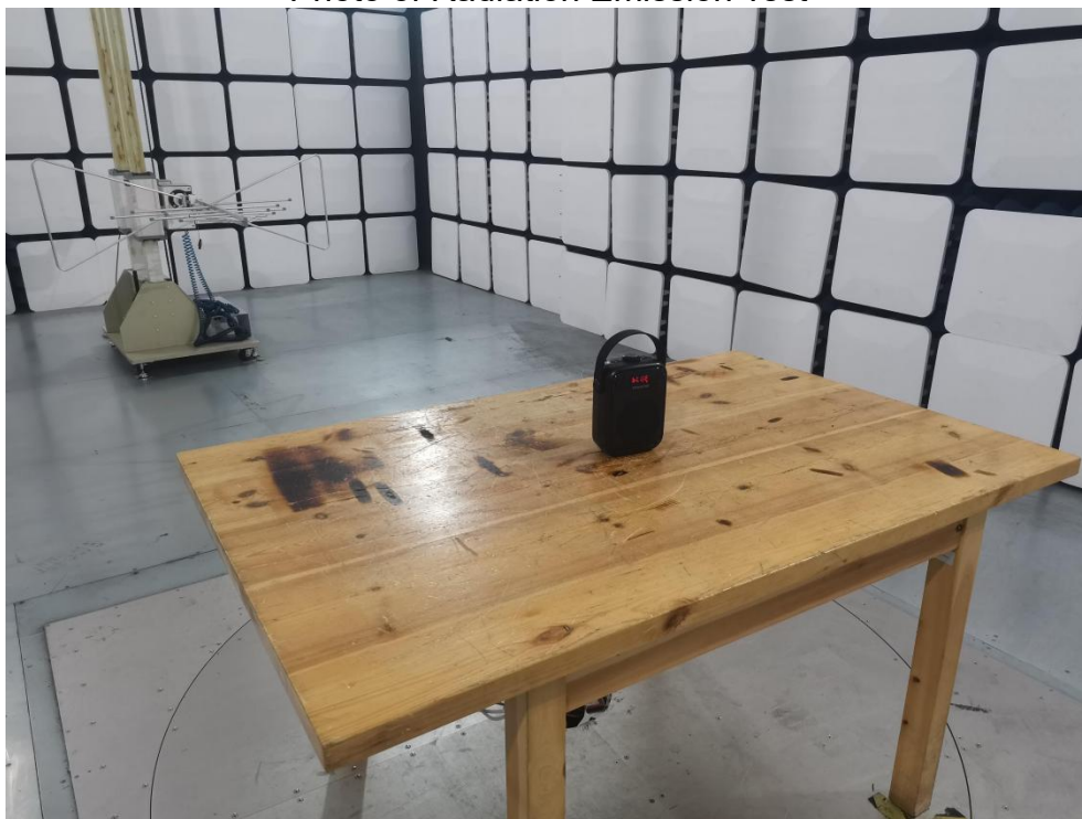
Photo of Radiation Emission Test
