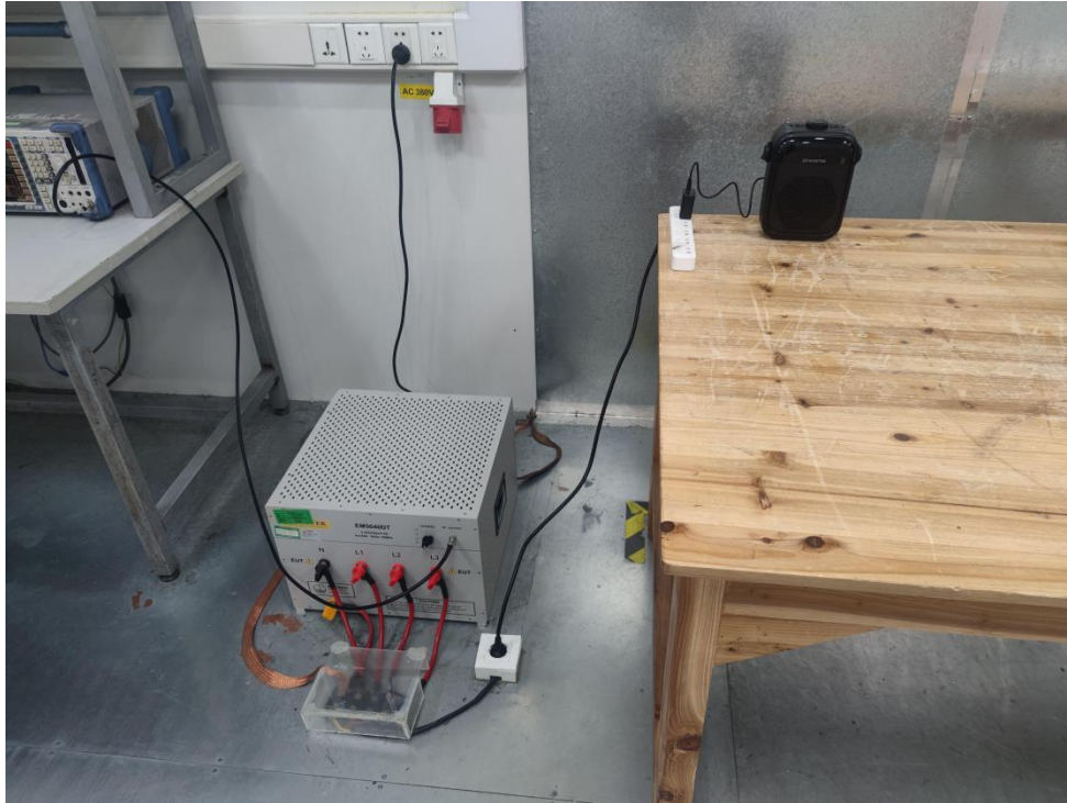
Photo of Conducted Emission Measurement
