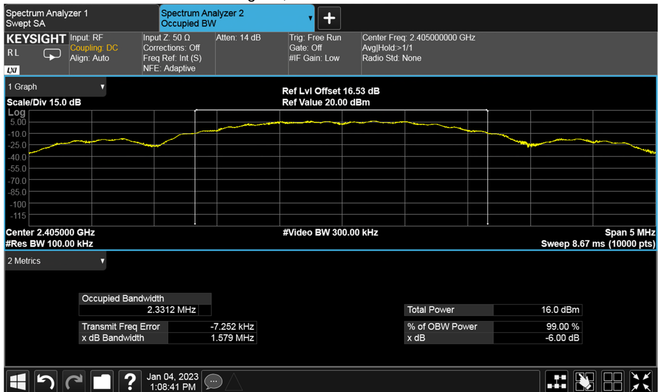
Plot for 6 dB Bandwidth Result (MHz)
