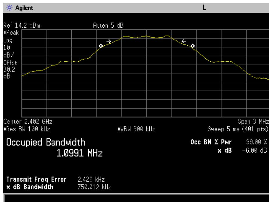
**6 dB and 99% Occupied Bandwidths at 2442 MHz – BLE**
