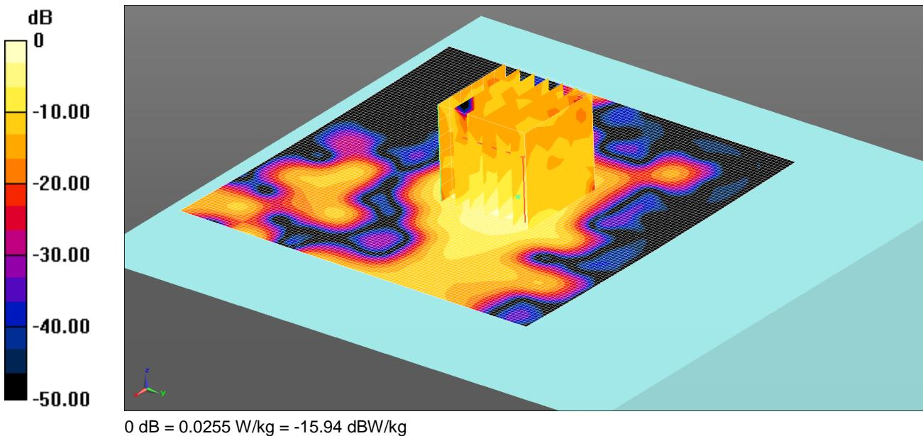
Communication System: UID 0, WLAN 802.11 (0); Frequency: 2437 MHz; Duty Cycle: 1:1
