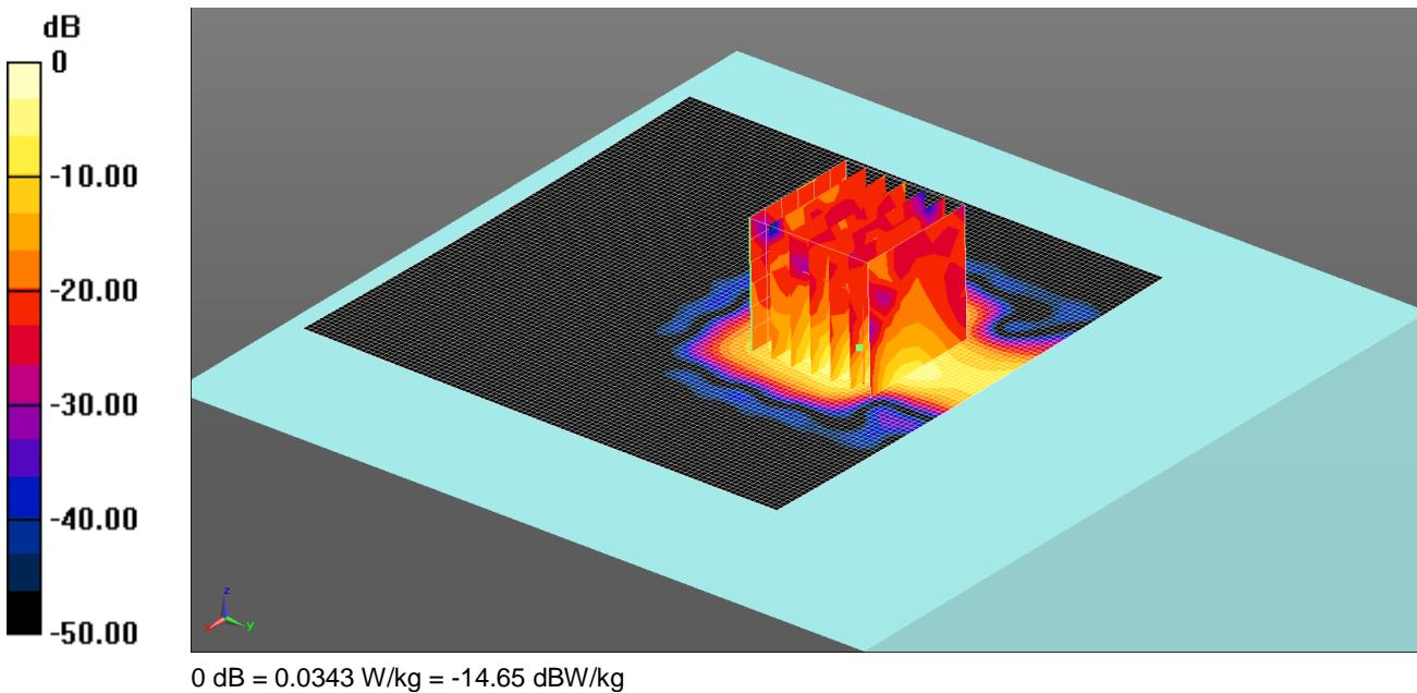
Communication System: UID 0, WLAN 802.11 (0); Frequency: 2412 MHz; Duty Cycle: 1:1
