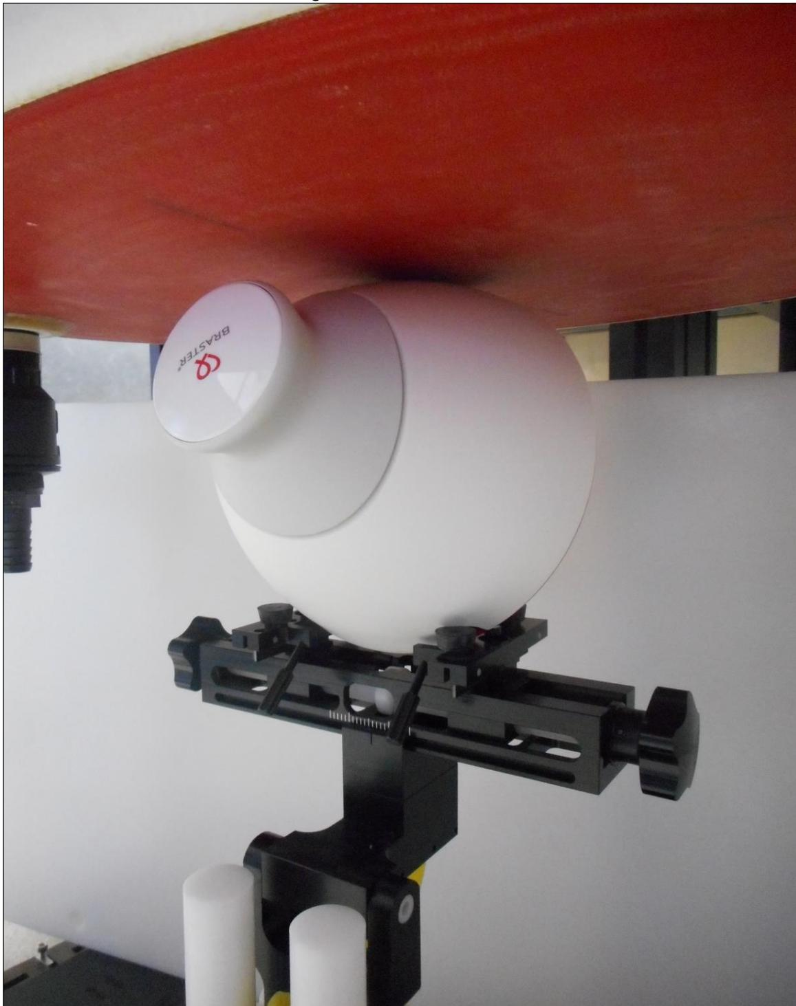
PHT/005: Position 4 of DUT Facing Phantom at 0mm
