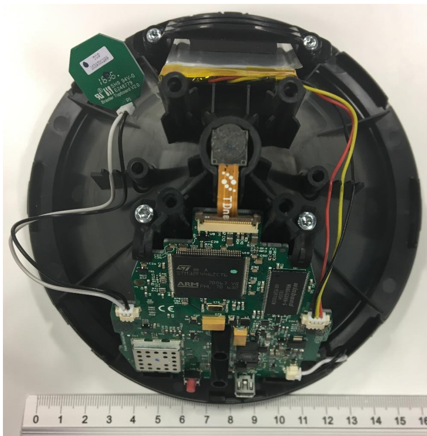
Fig. 6 View of BRA-1.0 without housing
