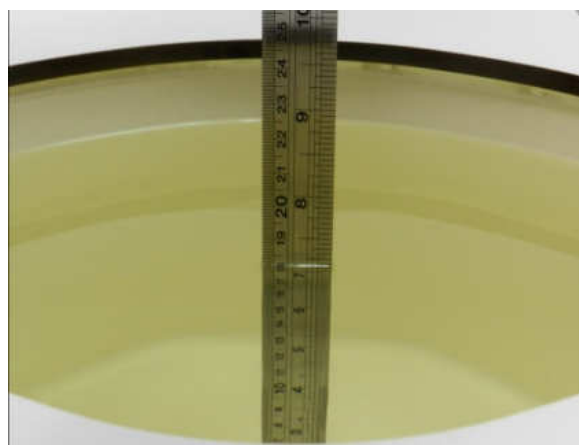
Fig 10.2 Photo of Liquid Height for Body SAR
