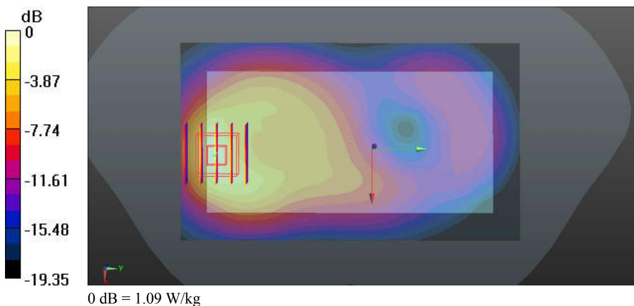
**13\_LTE Band 4\_20M\_QPSK\_1RB\_49Offset\_Back\_10mm\_Ch20175**
