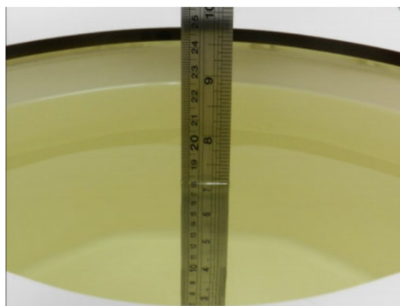
Fig 10.2 Photo of Liquid Height for Body SAR
