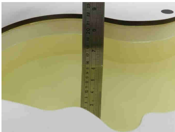
Fig 10.1 Photo of Liquid Height for Head SAR
