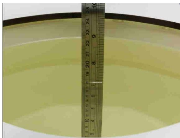
Fig 10.2 Photo of Liquid Height for Body SAR
