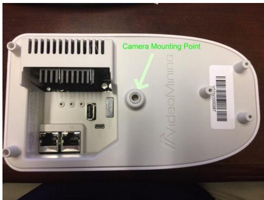
The threaded camera mount connection, threads into the top side of the VideoMining OmniSensr v2. This side is found by locating the corresponding camera thread port by the VideoMining logo.
