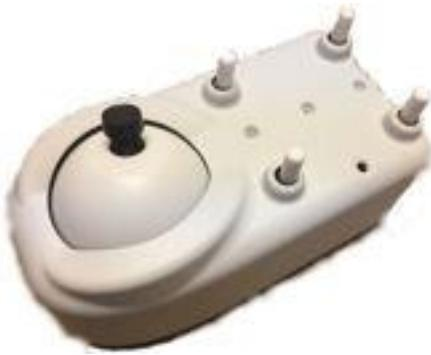
The VideoMining OmniSensr v2, is a multifunction camera and sensor device that is mounted in various locations throughout the clients' location. The standard camera mounting system:
