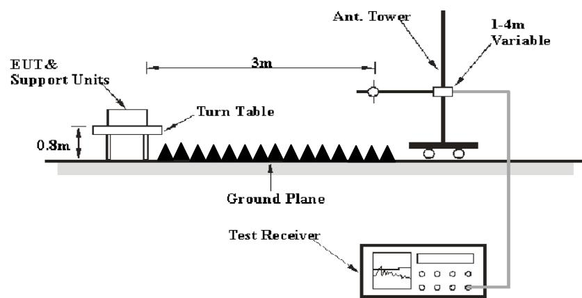
The radiated emission tests were performed at the 3 meters chamber test site, using the setup accordance with the ANSI C63.4-2014. The specification used was the FCC Part 15.109 Class B limits.
