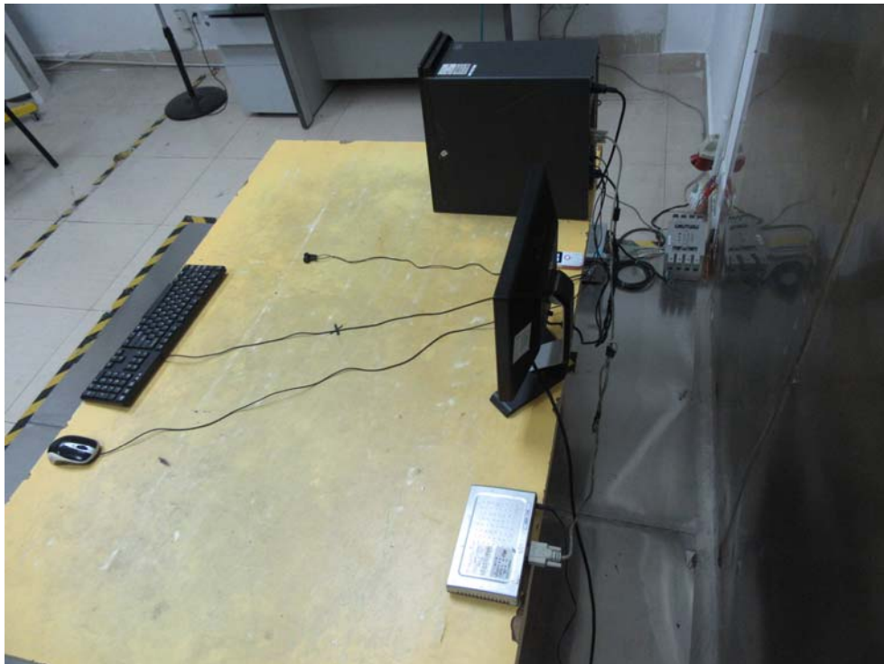
Conducted Emissions - Side View
