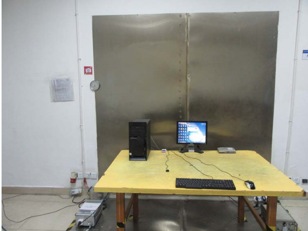
Conducted Emissions - Side View
