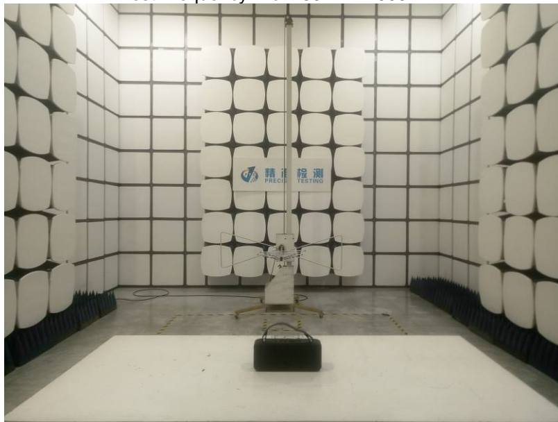
Radiated Spurious Emissions Test Frequency From 30MHz-1000MHz
