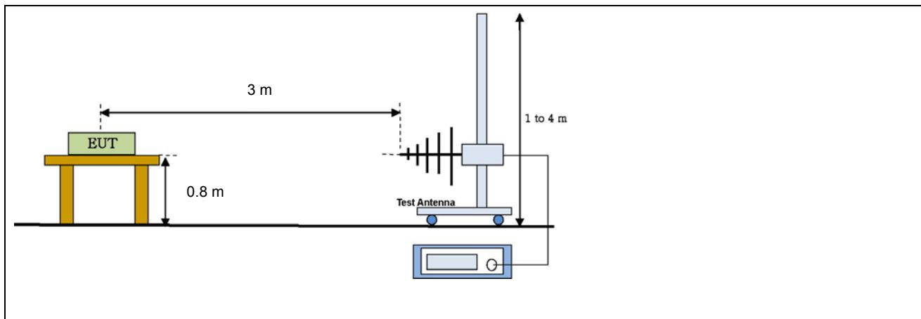
Radiated emission setup, Above 1 GHz
