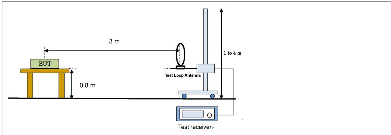
Radiated emission setup, Below 1 000 MHz
