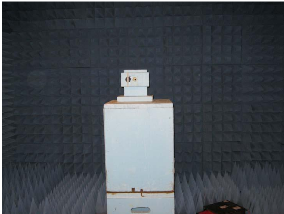
Radiated Emissions above 1 GHz – Position 2
