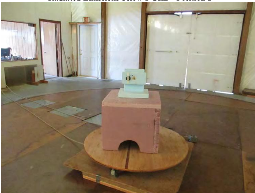
Radiated Emissions below 1 GHz – Position 2
