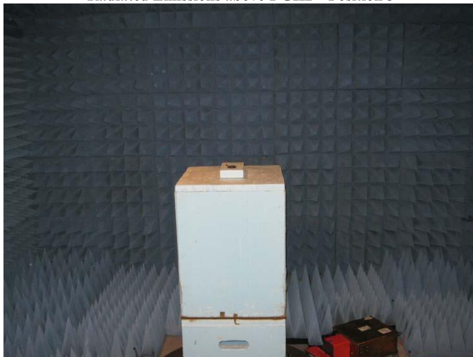
Radiated Emissions above 1 GHz – Position 3
