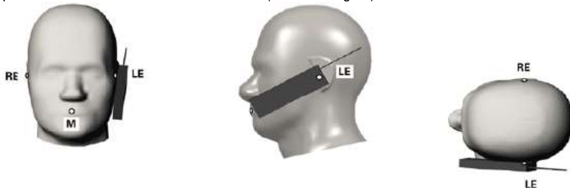
Fig. 11.3 Illustration for Cheek Position
