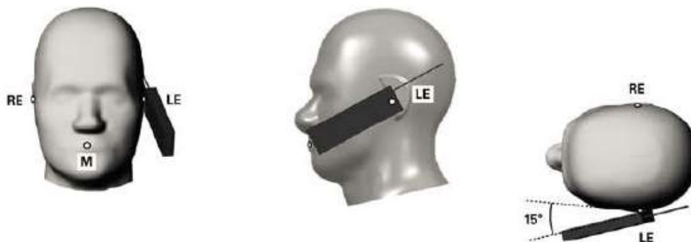
Fig.11.4 Illustration for Tilted Position
