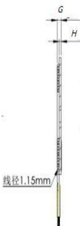
Note: 8MM(ref) high-temperature adhesive tape is wound around the wire outlet of the coil, and double-sided adhesive is attached to the back of the magnetic sheet.
