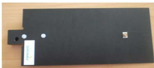
Figure 1 – MVG COMOHAC Validation Dipole
