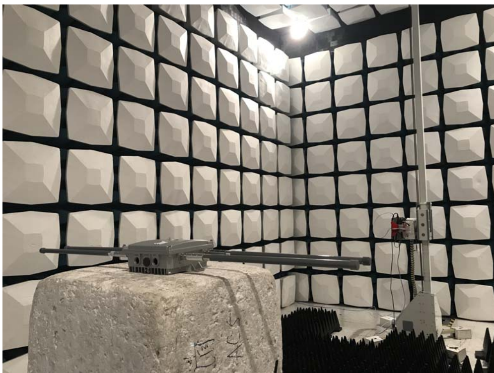
Description: Radiated Emission Test Setup for 1~18GHz
