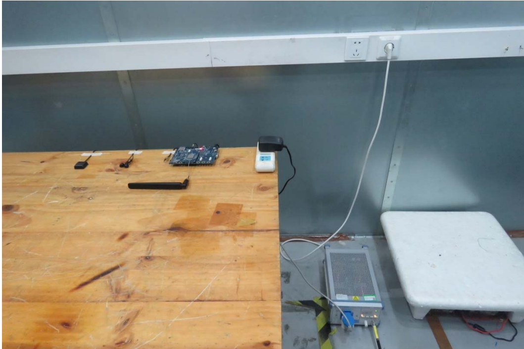
Picture 3: AC Power Line Conducted Emissions Test setup
