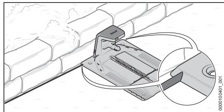
If the docking station has been positioned directly against a wall, it is also possible to install the connecting cord under the base plate. The connecting cord can be routed out of the base plate to the left or right.
