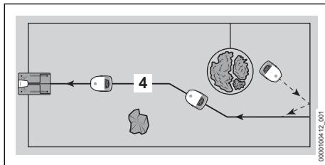
At least one guide wire (4) must be installed in the mowing area. A maximum of three guide wires can be installed.
