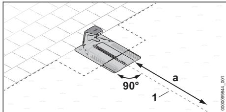
The docking station is at the edge of the mowing area. The adjacent area is navigable and the guide wire (1) can be routed in a straight line from the docking station into the mowing area over a length  $a = 6.6$  ft. (2 m).
