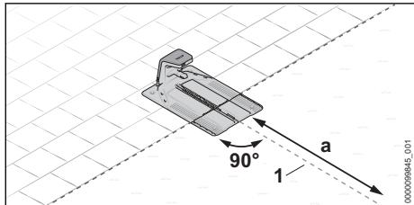
The docking station is partly in a navigable area and partly in the mowing area and the guide wire (1) can be routed in a straight line from the docking station into the mowing area over a length  $a = 6.6$  ft. (2 m).
