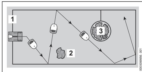
This iMOW® is a mulching mower, designed for autonomous, programmable lawn care. It mows the lawn in randomly chosen paths. During mulching, the grass clippings are further shredded in the mowing deck after cutting. They then fall back into the turf, where they decompose. It is necessary to route a perimeter wire (1) so the robotic mower can identify the boundaries of the mowing area.
