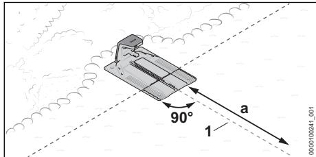
The docking station is partly in a bed and partly in the mowing area and the guide wire (1) can be routed in a straight line from the docking station into the mowing area over a length  $a = 6.6$  ft. (2 m).
