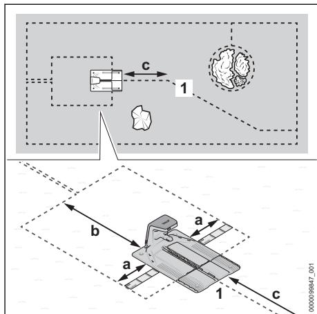
The docking station is positioned as an island in the center of the mowing area.
