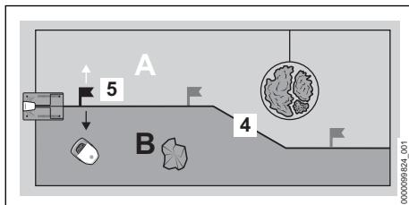
Up to three starting points (5) can be specified on a guide wire (4). The robotic mower can move specifically to the respective starting point and start mowing from there.
