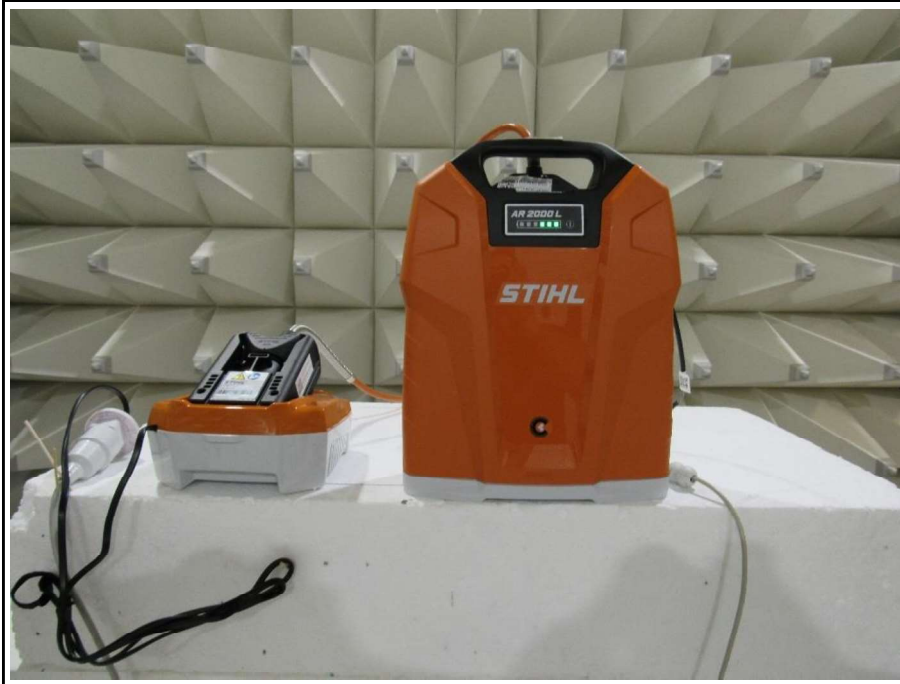
EUT test setup above 1 GHz
