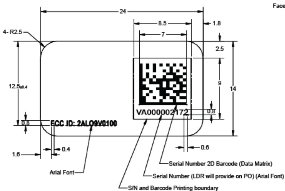
1. the dimension of the label are 24 mm by 14 mm. The rear of the EUT measures 74 mm by 34 mm. Due to the size of the EUT, the FCC compliance statement is included in the instruction manual.
