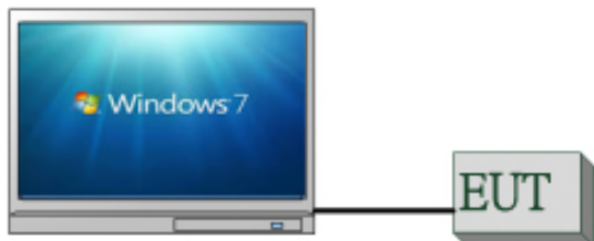
Fig. 2-2 Conducted Emission (AC Power Line) Configuration
