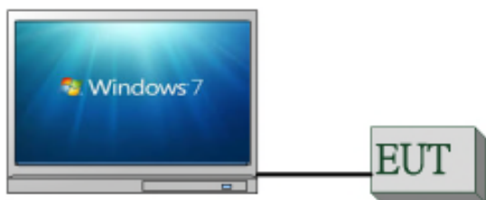
Fig. 2-2 Conducted Emission (AC Power Line) Configuration
