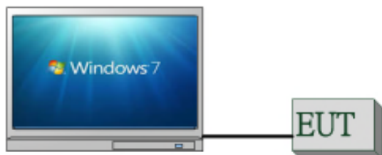
Fig. 2-2 Conducted Emission (AC Power Line) Configuration
