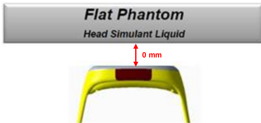
Fig-4.1 Illustration for Smart watch Setup
