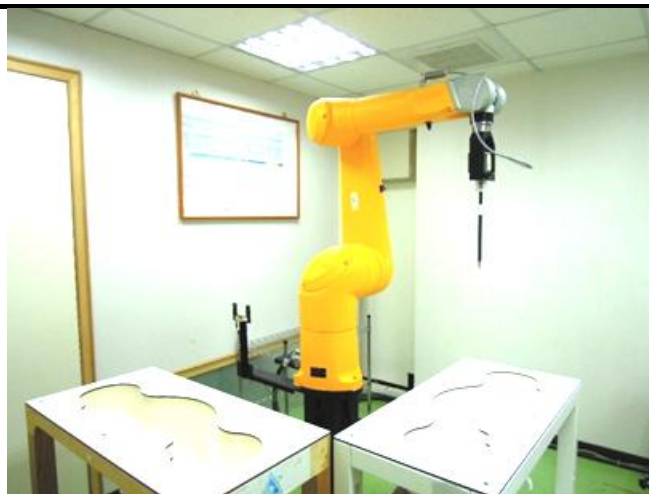
Fig-3.2 SPEAG DASY52 System
