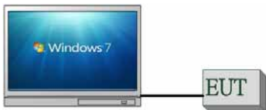
Fig. 2-2 Conducted Emission (AC Power Line) Configuration
