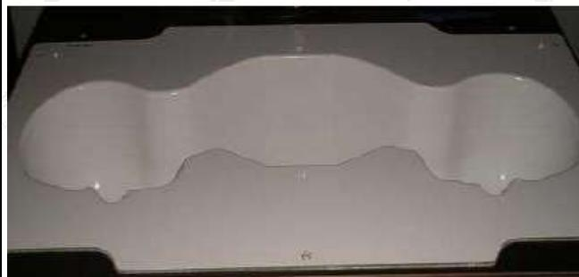
The bottom plate contains three pairs of bolts for locking the device holder. The device holder positions are adjusted to the standard measurement positions in the three sections. A white cover is provided to tap the phantom during off-periods to prevent water evaporation and changes in the liquid parameters. On the phantom top, three reference markers are provided to identify the phantom position with respect to the robot.
