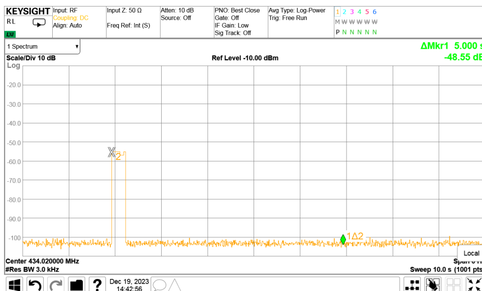
Plot 7.1.1 Transmitter shut down test result
