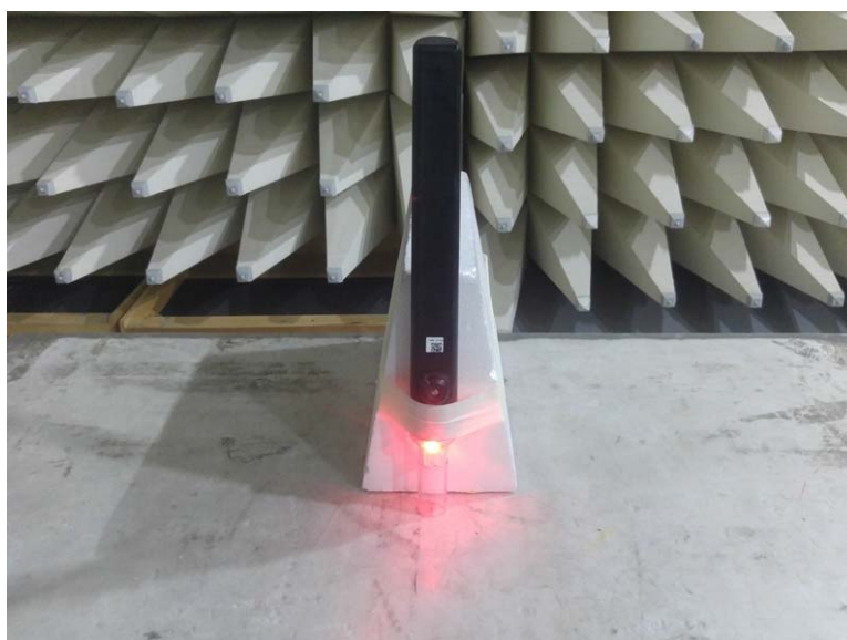
Photograph 8.1.3 Setup for radiated emission measurements, EUT close view
