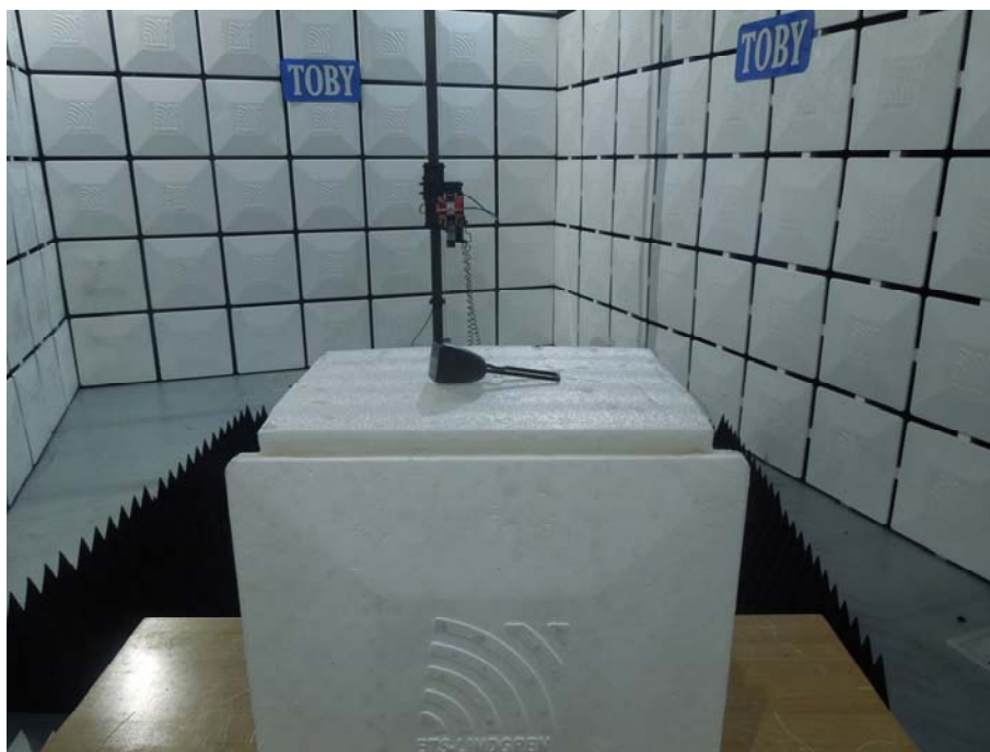
Photo of Setup for Radiated Emission (Above 1 GHz) -6 inch Ant.
