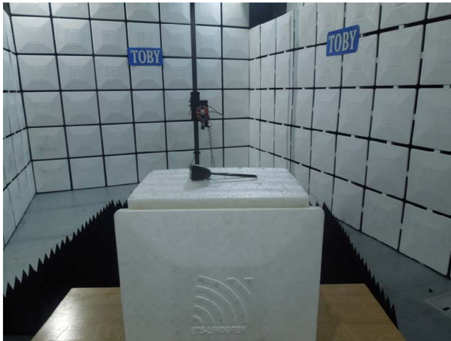
Photo of Setup for Radiated Emission (Above 1 GHz) -6 inch Ant.
