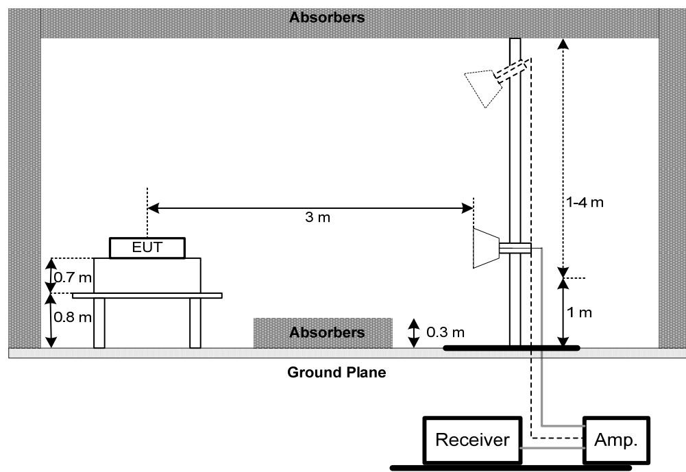
(C) For radiated emissions below 30MHz
